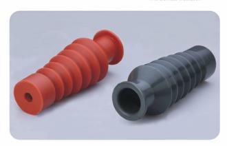
Bushing Boots are non-tracking elastomeric insulating boots which are used in conjunction with terminations. They fit over the bushings of switchgear, insulating the area between the cable connector in either right angled or straight bushing connections. They are designed to enhance the phase-to-phase and phase-to-earth insulation. The boots can be used up to 25 KV application & protect against flashover or surges induced in switchgear & transformer boxes.
