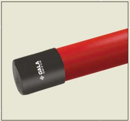
Cold Shrink End Cap is used to seal the ends of all types of Cables & protect from ingress of water / moisture. The caps are manufactured from high quality EPDM Rubber compatible with most commonly used Cable Jackets i.e. XLPE, PVC, PILC or Rubber Sheathed Cable.
